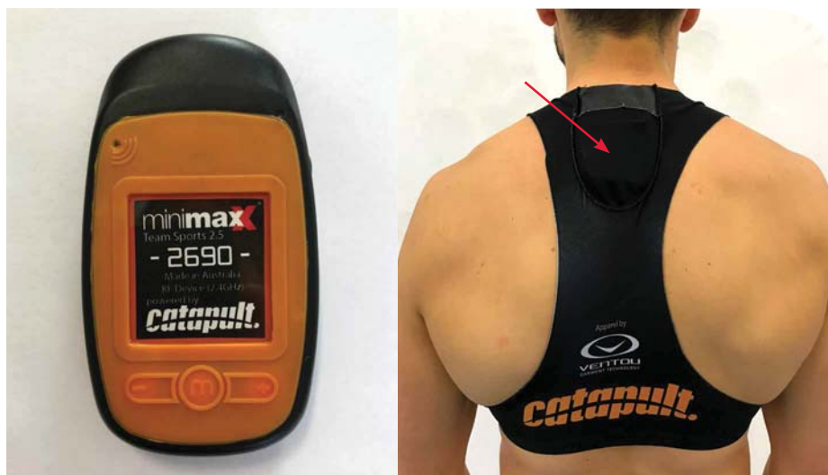
Figure 1. Portable MEMS device (L) and fast bowler wearing a bespoke neoprene vest (R). The red arrow indicates unit placement, between the scapulae, within a custom-made pouch as part of the bespoke neoprene vest
